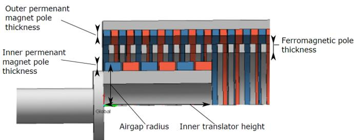
Figure 7: Main magnetic gear parameters
