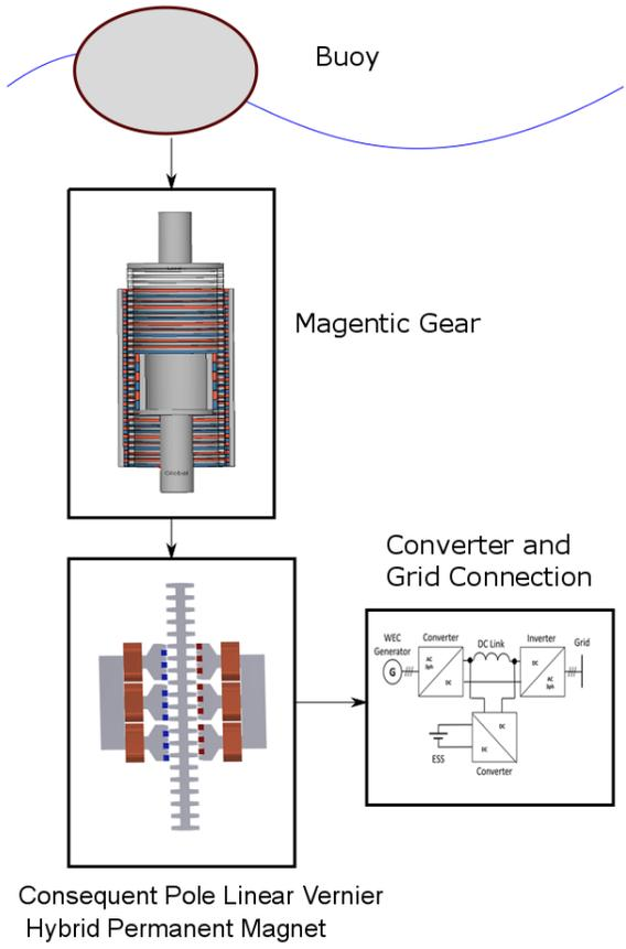
Figure 6: Combined system layout
