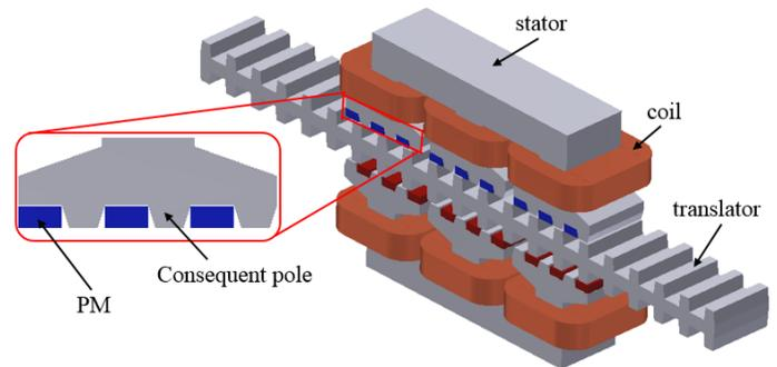
Figure 1: Configuration of CPLVHPM machine
