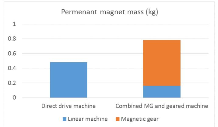
Figure 9: Permanent magnet mass of designs
