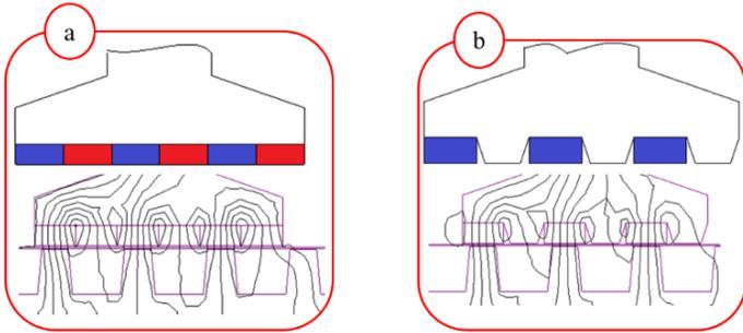
Figure 2: The effect of consequent poles on leakage flux
