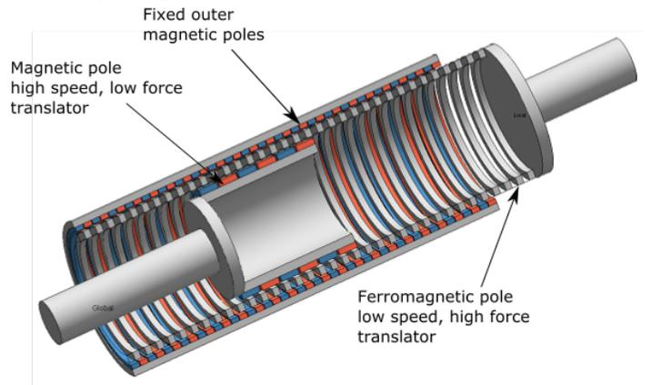
Figure 3: Magnetic gear topology
