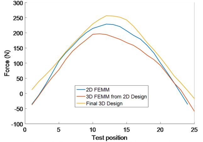
Figure 5: Forces on high speed, PM pole translator
