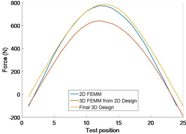
Figure 4: Forces on low speed, ferromagnetic pole translator
